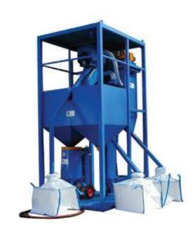
The air wash action can be regulated to control the size of the reusable abrasive. Dust and non-usable (too fine) abrasive are automatically discharged and collected in big bags or extracted by the separate filter. The cleaned abrasive will fall into the abrasive silo and is ready to be stored into big bags or into blast vessels.
