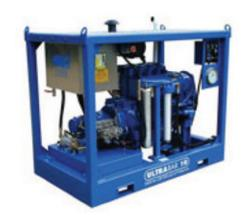
are manufactured from stainless steel as standard. The in-line valve arrangement prevents the adverse effects of cyclic stress within the headblock, while allowing all working components to be easily removed on site for service. Solid ceramic plungers extend the life of the self adjusting plunger seals. The UB-range of UHP pumps includes design features that allow seals and valves to be monitored without tools and maintenance on individual cylinders.
