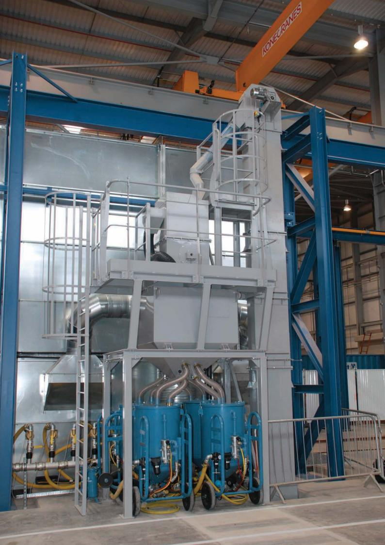
Our method of grit reclassification is proven to extend the life of dust extraction filter cartridges.
